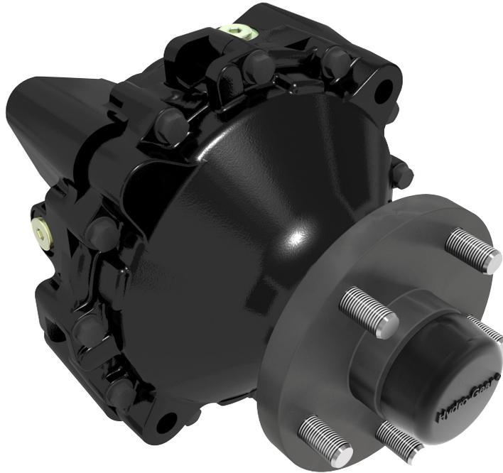
**Introduction** The HGM-H from Hydro-Gear® is a new Low Speed High Torque (LSHT) wheel motor utilizing piston technology. Available in 15 & 18 cu. in displacement, the HGM-H is designed for applications where high output torque is needed. With its dual stage planetary gear reduction and heavier axle, the HGM-H offers many features not found on typical geroller LSHT motors. The HGM-H is covered by a full commercial warranty.
