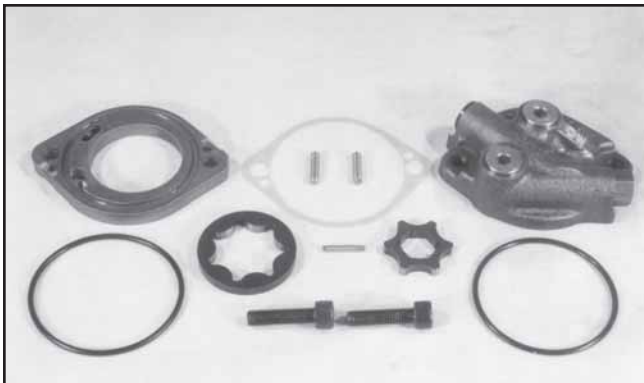
BDU-21L/A CW Charge Pump Components
