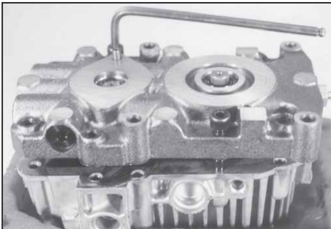
BDU-10S Center Section Removal
