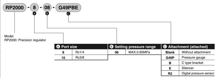
Note 1: If the port size Rc1/2 is required, use a piping adapter set (model no.: A400-15).
