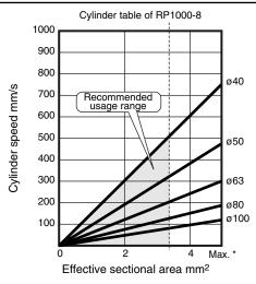
This cylinder table shows available range according to air supply / exhaust flow rate of precision regulator and required consumption flow rate at cylinder PUSH/PULL.
