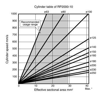
This cylinder table shows available range according to air supply / exhaust flow rate of precision regulator and required consumption flow rate at cylinder PUSH/PULL.
