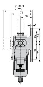
\*1. Dimension when digital pressure sensor assembled.
