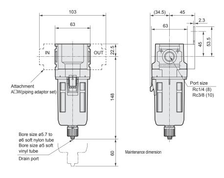
Attachment C type bracket (-BW) Part model no.: B320
