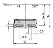
Pressure gauge attached optional dimensions table
