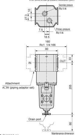
Port size Rc3/4 (20) Rc1 (25) • Attachment C type bracket (-BW) Part model no.: B620
