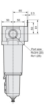
• Attachment C type bracket (-BW) Part model no.: B820
