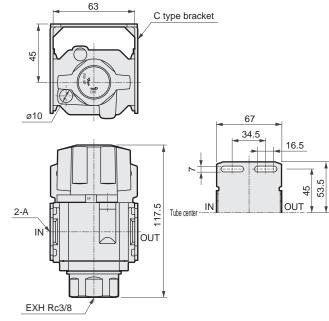
The C type bracket is attached at shipment. C type bracket and piping adaptor set can not be used together.
