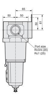
• Attachment C type bracket (-BW) Part model no.: B820
