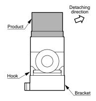
(3) When mounting a manifold, the project on the bracket into the other bracket's slot.
