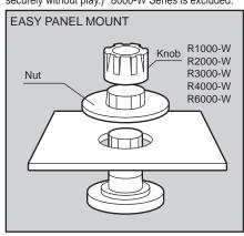
Note:Install the nut before installing the knob. (With the R2000-W, the nut is removed without removing the knob.)
