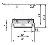
Pressure gauge attached optional dimensions table
