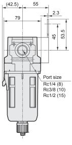
Attachment C type bracket (-BW) Part model no.: B420
