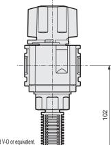
• Silencer (-S) Part model no.:SLW-10A The silencer is attached at shipment. The silencer is made of flame resistance resin UL94 Standard V-O or equivalent. Note that the element is not manufactured of flame resistance resin.
