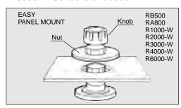
Note: Install the nut before installing the knob. (With the R2000-W, the nut is removed without removing the knob.)
