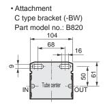
Pressure gauge attached optional dimensions table
