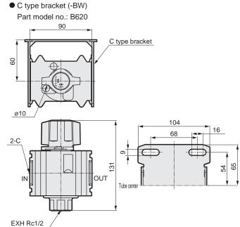
The C type bracket is attached at shipment.
