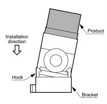
(2) To remove the product, tilt it slightly to the side, and release one hook.
