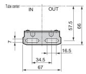
Pressure gauge attached optional dimensions table
