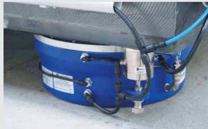
Air spring for test bench
