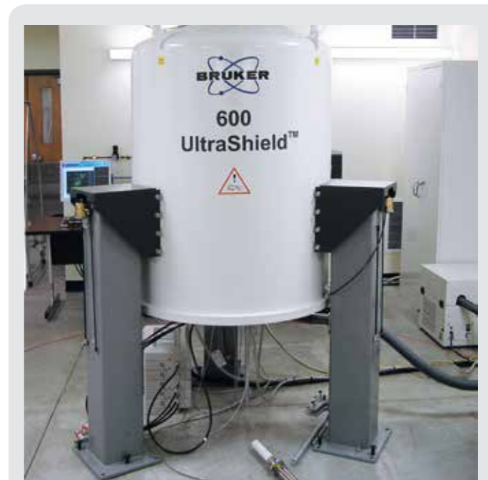
600 MHz NMR on PAL18 gimbal air springs
