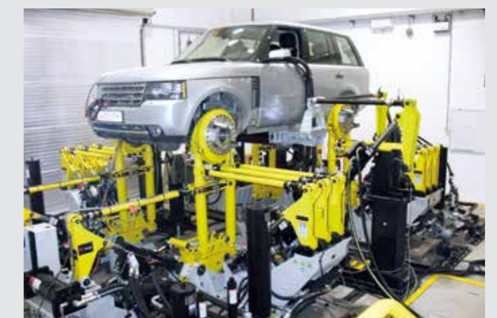
Chassis dynamometer on a vibration-isolated foundation
