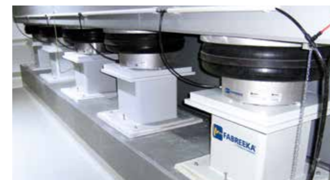
RLA isolation with RLA air springs on supports (with levelling)
