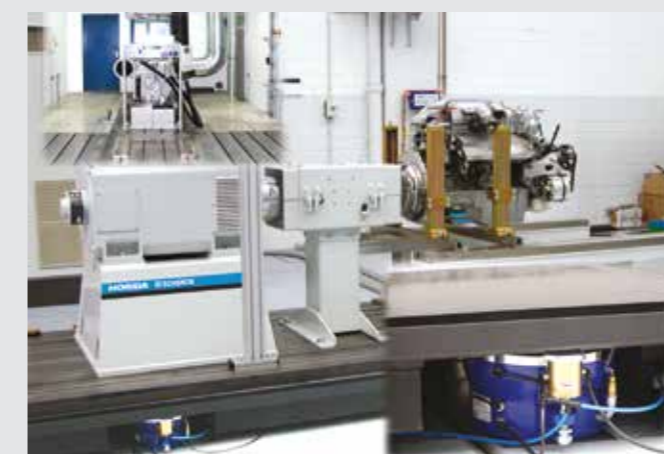
Motor test bench on PAL
