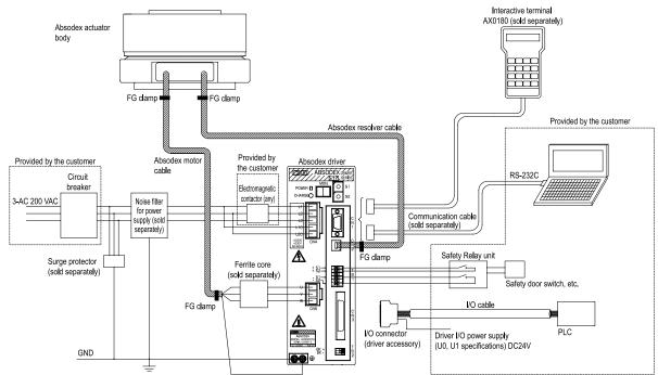
To comply with CE marking requirements, the following parts as well as overcurrent protection, short-circuit protection, and other components are required. In addition, the driver must be installed inside the switchboard. For details on how to select these devices and how to install and wire these devices, refer to the instruction manual or the technical information (ABSODEX AX Series TS Type/TH Type Technical Information).
