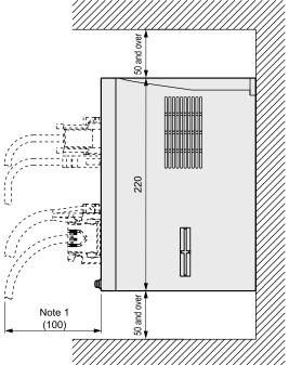
Note 1) Determine a dimension that is more than sufficient for the cable that you are using.
