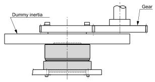
[Fig. 5] Dummy inertia attachment example 3
