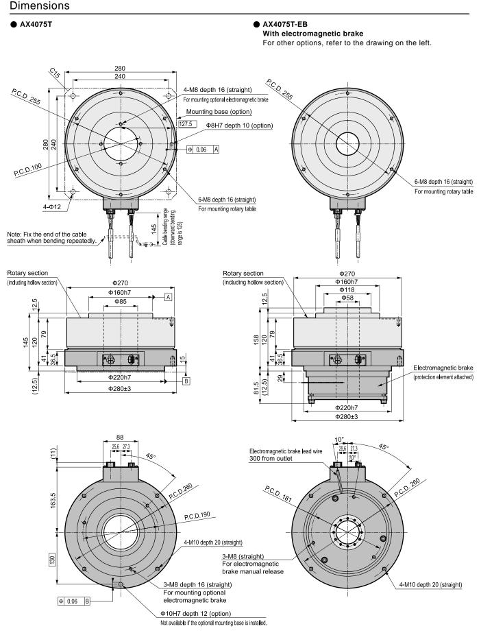
Note 1) The actuator's origin may differ from that in the dimensional drawing. The origin offset feature enables you to set the origin to any position you choose.
