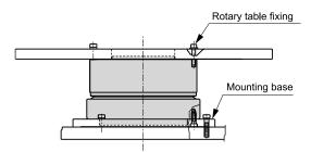
Gain must be adjusted based on load table size, etc. Even when the Absodex is not directly installed, it should be installed on a highly rigid frame. [Fig. 2]
