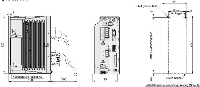
Note 1) Mounting pitch is different from the conventional models (AX9000GS/AX9000GH).
