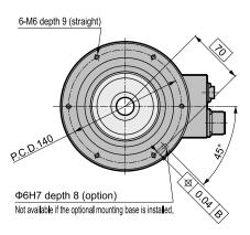
Note 1) The actuator's origin may differ from that in the dimensional drawing. The origin offset feature enables you to set the origin to any position you choose.
