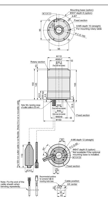
Note 1) The actuator's origin may differ from that in the dimensional drawing. The origin offset feature enables you to set the origin to any position you choose.
