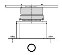
8 When extending the output shaft, refer to the references given in Table 1 for the extended shaft's diameter and length. In addition, add dummy inertia by using Fig. 3 as a reference.
