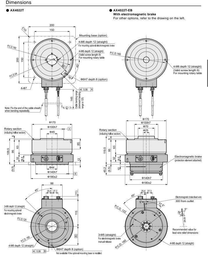
Note 1) The actuator's origin may differ from that in the dimensional drawing. The origin offset feature enables you to set the origin to any position you choose. AX4000T
